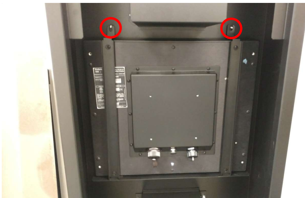
Figure 18 - Straps Inserted. Attach 2 Nuts to Secure
